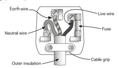
The wire coloured BLUE is the NEUTRAL and must be connected to the terminal marked N or coloured BLACK.
