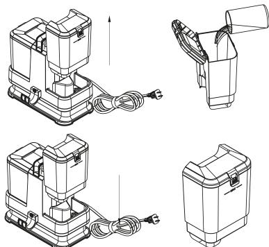
**STEP 1:** Remove the clean water tank by lifting it away from the spot cleaner main unit.
