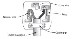
The wire coloured BROWN is the LIVE wire and must be connected to the terminal marked L or coloured RED.
