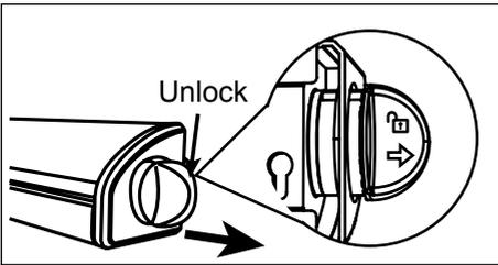
**STEP 8:** Turn the locking mechanism (6) clockwise to tighten the lines fully and then push the side locking mechanism in to secure in place.
