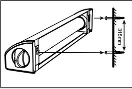
**STEP 5:** Install the fixing hooks (4) by making four holes onto a suitable surface opposite to the retractable clothes line, checking that it is no more than approx. 4 metres away. The fixing hooks must be installed at the same height as the washing line bar (5) and ensure that the holes created align with the fixing hook holes.
